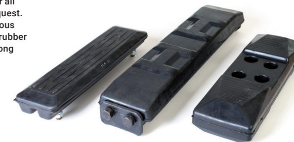
NTP rubber pads are available in three different versions: Chain-on which is replacing the steel shoe and bolted directly on the chain, Clip-on is attached with clips to the existing shoe, and Bolt-on which is bolted through pre-drilled holes in the steel shoe.
