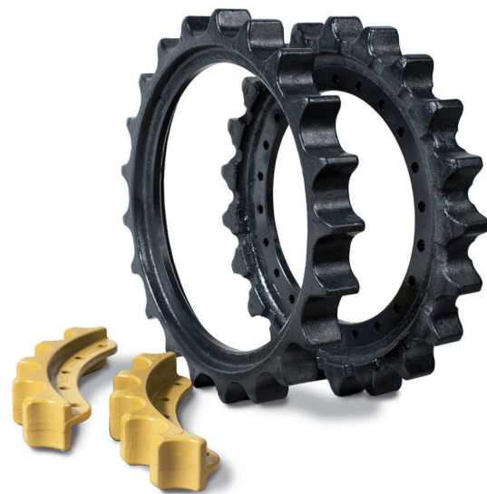
Sprockets are available as welding rim and bolt-on for excavator and bolted segment for bulldozers. The sprocket surface is heat treated in one shot in order to get the same hardness in continuity in every tooth.
